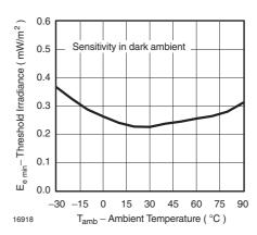
Figure 10. Sensitivity vs. Ambient Temperature
