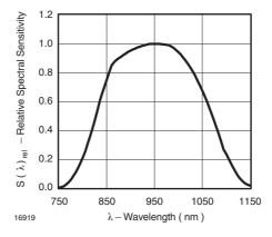
Figure 11. Relative Spectral Sensitivity vs. Wavelength
