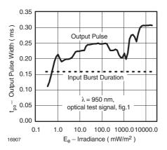
Figure 2. Pulse Length and Sensitivity in Dark Ambient
