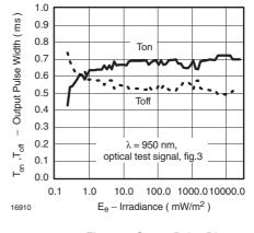
Figure 4. Output Pulse Diagram
