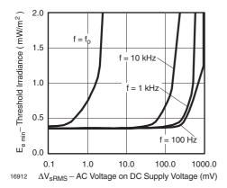
Figure 7. Sensitivity vs. Supply Voltage Disturbances
