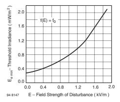
Figure 8. Sensitivity vs. Electric Field Disturbances
