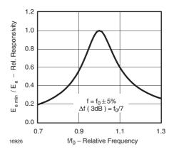
Figure 5. Frequency Dependence of Responsivity
